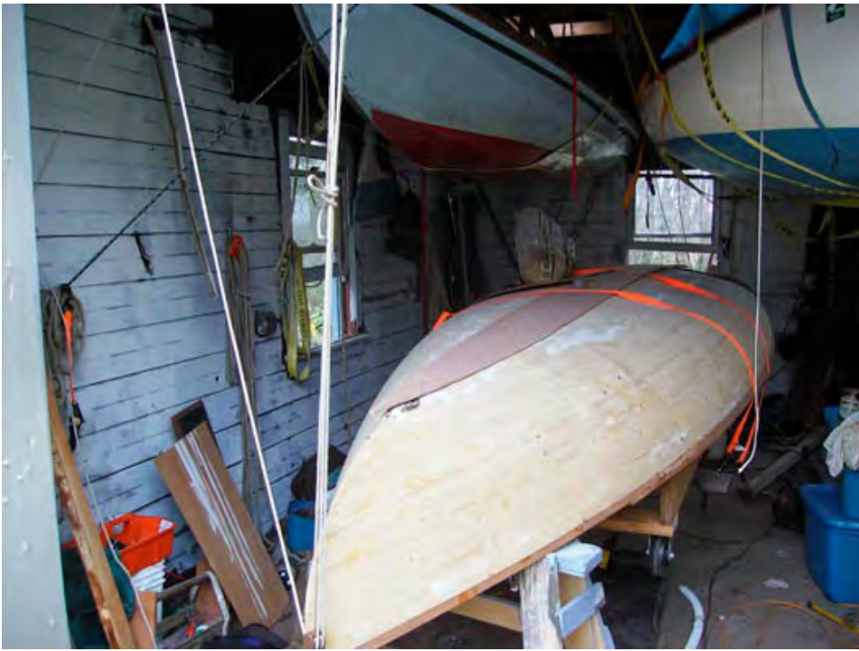
A temporary garboard is being fitted here. This, along with a temporary transom, keel batten and nose cone, form a landing for the first layer of planking.
