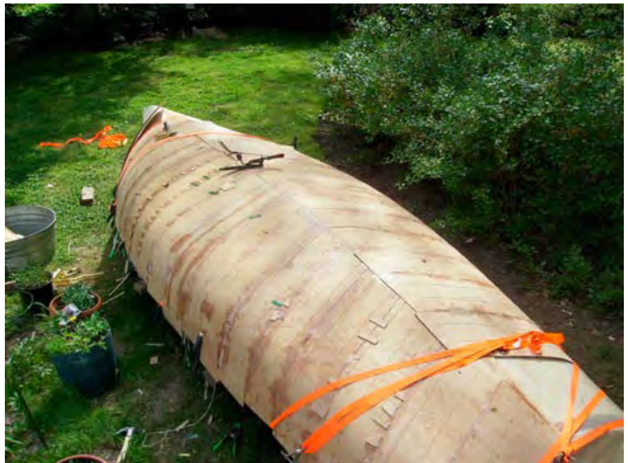
The first layer of planking nearly complete.
