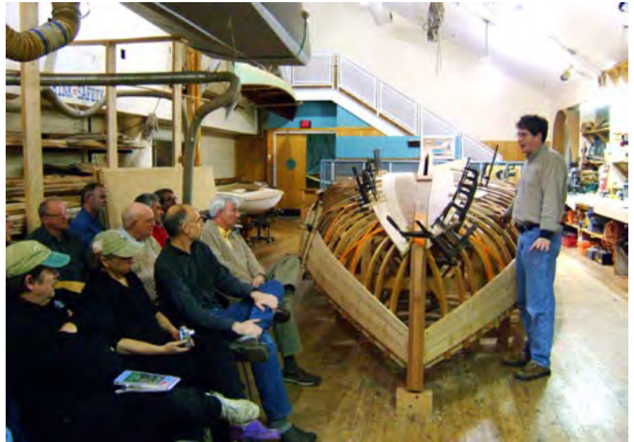
John discusses the construction of the A-cat SPYDER. In addition to her visible diagonal strapping, her interior is to be fitted with overlapping rigid structures to minimize twist.
