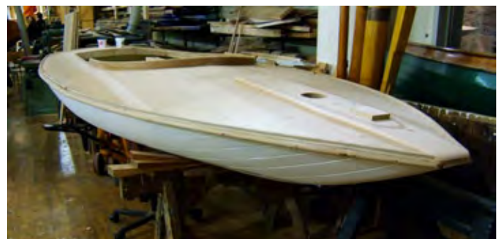
The sneakbox showing its distinctively planked shallow hull.
